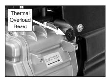
Figure 8. Thermal overload reset.
